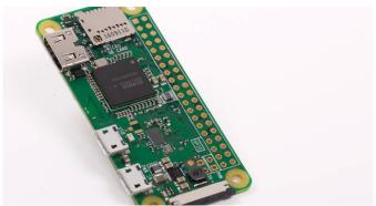
The Pi Zero W carries the same specifications as its predecessor on a slim single-sided board, namely a 1GHz single-core Broadcom BCM2835 CPU, 512MB RAM, mini-HDMI port, micro-USB port and a HAT-compatible 40-pin header. Wireless connectivity comes through the addition of a Cypress CYW-43438 chip, the same found in the Raspberry Pi Model B.
