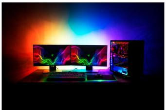
The Chroma HDK features the same Synapse 3 controlled RGB LEDs found in the company's PC systems and peripherals. The actual kit consists of 2 LED strips (each with 16 RGB LEDs) together with a base module offering 4 lighting channels. Customers can also add more lighting through a Lightpack Extension Kit packing two RGB LED strips and extension cables.
