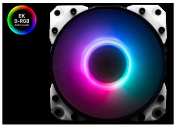
The extended range PWM fans are available in 120 and 140mm sizes, and promise not only a quieter environment but also prevent dust build-up in idling PCs, extending fan lifespans. To determine when to stop spinning the fans have a PWM curve set so if the PWM duty cycle is below 25-30% PWM (depending on motherboard model) the fan simply stops spinning.
