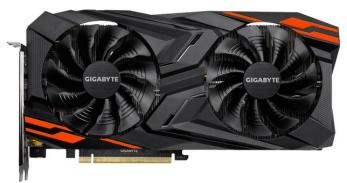
The Vega 64 features processors clocked at 1276 MHz base and 1560 MHz base, making it slightly faster than the 1247 MHz base and 1546 MHz boost clocks of the reference card. Allowing such speeds are a dual-fan Windforce 2X cooler, a "well rounded thermal solution" consisting of 5 heatpipes in direct contact with the GPU and a copper plate with an extra heatpipe on the back of the card.
