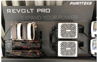
The Revolt Pro is described by the company as "the first expandable power supply." customers can connect a Revolt Pro with any other power supply to combine the total power output. In addition the secondary PSU acts as a backup power source via integrated redundancy feature.
