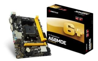
Being aimed at customers on a budget, the A68MDE features a single PCIe x16 slot for discrete graphics together with another PCIe slot for x1 devices. It has two DIMM slots for dual-channel memory, and supports up to 32GB DDR3 RAM overclocked up to 2600MHz.
