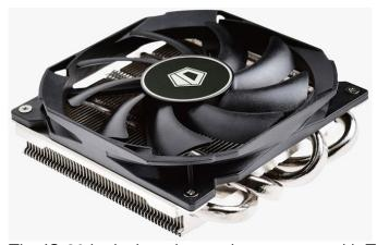
The IS-30 is designed to cool processors with TDPs up to 100W, meaning it can handle 8-core unlocked processors such as the Intel Core i9-9900K or AMD Ryzen 2700X. It features a cooling design with four copper heat pipes, multiple aluminium fins and a 92mm PWM fan spinning at 800-3600RPM to create airflow reaching up to 40 CFM.
