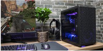
The MasterBox Q500L measures 386 x 230 x 381mm, with an unpopulated mass of 3.83kg, yet can fit graphics cards of up to 360mm even with an ATX power supply. In total it supports up to 7 slots, fitting up to four 2.5-inch devices in two combo bays, one 120mm rear fan (included), two 120 or 140mm fans in the top (or up to 240mm radiator with 35mm depth) and two 120mm fans in the bottom. CPU cand PSU clearance are 160 and 180mm respectively.
