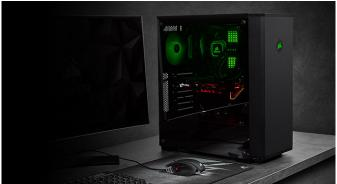
The chassis weights 6.1kg and measures 418 x 210 x 450m, meaning it fits Mini-ITX, Micro ATX or ATX motherboards, as well as GPUs up to 330mm long, CPU coolers 160mm tall and 180mm ATX PSUs. It includes a single 120mm RGB fan, and can fit three 120mm fans or one 140mm fan in the front, two 140mm fans in the top and one 120mm fan in the rear. Customers can also opt for liquid cooling, with space for a radiator measuring up to 360mm.
