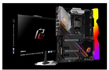
The two motherboards carry built-in lighting and RGB LED headesers, as well as a "beautifully designed" pre-installed I/O shield allowing more space for fitting tolerances. Customers can even adjust the shield during installation in order to fit the chassis perfectly. The two boards also include XXL aluminium alloy heatsinks, dual full coverage M.2 SSD heatsinks, 60A power chokes and a Dr. MOS design to ensure solid performance during overclocking.
