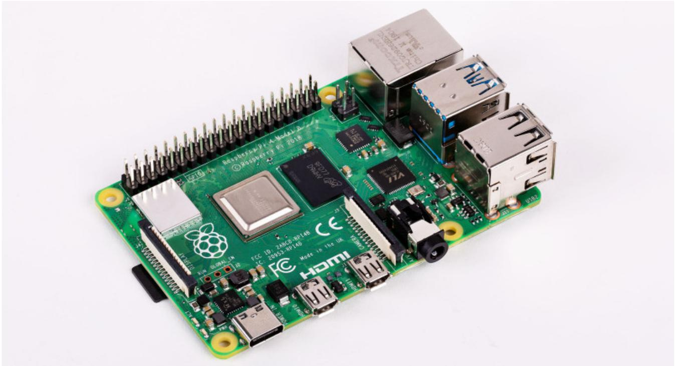
The Raspberry Pi 4 carries a 1.5GHz quad-core Broadcom processor (up from 1.4GHz in the previous model), a 500MHz VideoCore VI GPU (up from 400MHz) and up to 4GB LPDDR4 RAM. The result, the makers claim, is a tiny machine able to handle 4K 60fps video through the support for HEVC video, as well as dual-monitor support via dual micro-HDMI ports.
