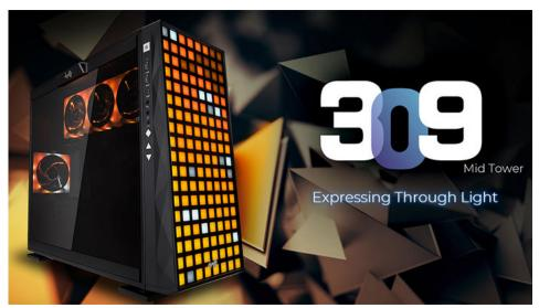
The company claims the front panel design is "inspired by the beauty of stained glass," which is perhaps a bit of a stretch. That said, customers can program the front panel LEDs via GLOW 2 software complete with customisable functions, a creator mode for own pixel art installations and 12 built-in lighting effects. The chassis even has a built-in mic, allowing the LEDs to react to sounds.
