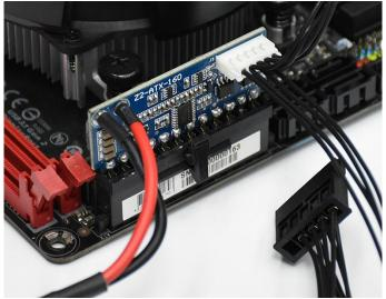
Small power supply maker PicoBox presents a PC PSU series measuring just 56mm-- the Z2, a PSU packing all components in a compact board customers can set on top of the motherboard 24-pin ATX connector.
