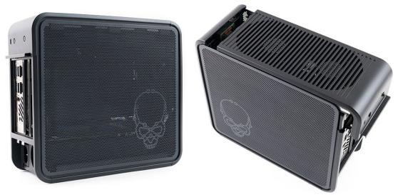
Allowances to fit regular GPUs make Ghost Canyon, also known as the Intel NUC 9 Extreme Kit, larger than other products in the Intel mini-PC range. In fact, it is more of a mini-desktop machine, if anything else. Intel is still to fully detail this latest NUC iteration, but does say it is powered by 9th gen Core H series processors ranging from Core i5 to Core i9, including a high-end Core i9 in an unlocked SKU.
