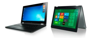
The IdeaPad Yoga is not just an ultrabook with a screen that flips over like a spiral-bound book-- it is also the first Windows 8 tablet from the company. It has a 13.3" 1600x900 multi-touch display, weighs around 1.47kg, is 16.9mm thick and will carry a "next-generation" (Ivy Bridge) Intel Core processor.
