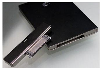
Part of the SATA 3.2 Revision, USM Slim trims the port to 9mm (down from 14.5mm) in order to allow integration with thinner devices.
