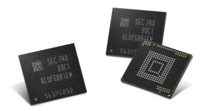
The storage components consist of eight 64-layer 512Gb Samsung V-NAND chips paired with a controller chip. The result is double the density of the previous 48-layer V-NAND-based 256GB eUFS, while taking the same amount of space within a device. Also included are a power management system minimising energy consumption and a faster mapping process for the conversion of logical block addresses to those of physical blocks.
