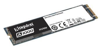
The single-sided M.2 2280 (22 x 80mm) format makes the A1000 ideal for notebooks, as well as systems with limited space. The drive features a gen 3.0 x2 interface, 4-channel Phison 5008 controller and 3D NAND flash, and promises x2 the performance of SATA SSDs with read/write speeds of up to 1500MB/s and 1000MB/s.
