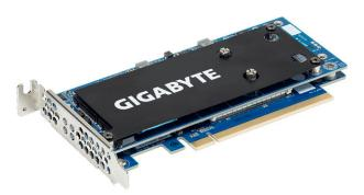
The CMT 4032 and 4034 have different minimum PCle slot requirements, depending on the number of drives supported. The CMT 4032 requires a PCle x8 (Gen3 x8 bus) connector slot, while the CMT 4034 needs a PCl x16 (Gen3 x16) slot. Both cards have the same low profile form factor, measuring  $150 \times 68.9 \, \text{mm}$ , and are compatible with M.2 type  $2280 \times 22110 \, \text{cards}$  measuring  $22 \times 80 \, \text{mm}$  or  $22 \times 110 \, \text{m}$ .
