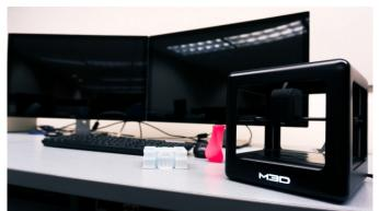
The Micro is a compact (it weighs 1kg) cube-shaped device promising reliable and low-power 3D printing. It prints objects using PLA and ABS plastics, as well as M3D filament spools, and reportedly prints out a teacup in all of an hour.
