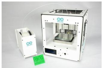
It features a 140 x 100 x 100mm print bed, allowing for the printing of items around the size of a large tea mug. Printing comes through Fused Filament Fabrication (FFF) via PLA filament, although Arduino says Crystal Flex, PLA Thermosense, TPU, PET, PLA Sand and PLA Flex filaments are also usable, if unsupported.
