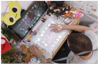
From a distance the Sprout looks like an All-in-One PC, only the keyboard is replaced by a mat and what looks like an desk lamp hangs on top of a 23-inch touchscreen. However the "mat" is actually a capacitative touch surface, and the "desk lamp" combines an Intel RealSense 3D camera, 14.6MP camera and a DLP projector beaming a work surface on the mat.
