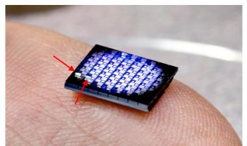
The extra-tiny (1 x 1mm!) computer is part of the "5 in 5," a collection of inventions and technologies IBM Research says "could change our lives in the next 5 years." It consists of a few hundred thousand transistors, an unspecified amount of RAM, a solar cell and an LED-based communications module. IBM adds it should be very cheap to produce, at around 10c apiece.
