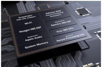
Current standalone VR headsets have had to make use of what are essentially repurposed smartphone processors. The XR1 claims to change the situation, since it is a platform powerful enough to handle such tasks while a fairly low price point. Admittedly the chipset does appear to be based on Qualcomm smartphone offerings, if tweaked with an emphasis on the processing of 3D XR tasks, such as audio/visual processing, user interaction and AI.
