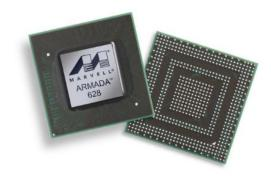
The Armada XP platform combines x4 1.6GHz Arm v7 compliant cores with a host of I/O peripherals (x4 PCI-e Gen 2.0 units, x4 gigabit networking ports, x16 Marvell Serdes lanes, multiple USB ports).
