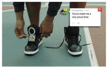
Shown off at the South by Southwest (SXSW) 2013 conference, the "Google Shoe" consists of an Adidas sneaker with an accelerometer, gyroscope, Bluetooth radio, custom-built microcontroller and a circular speaker grafted in the tongue.
