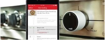
The Meld system consist of a motor-powered smart knob (replaces existing stove knobs), a thermometer one clips onto pots or pans and an obligatory smartphone app tying the two together. Essentially, the user sets a desired temperature on the app before the thermometer and the knob work in tandem via Bluetooth connectivity to maintain said temperature.
