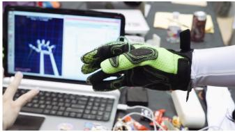
The right-handed glove is designed to be unobtrusive, being wireless and, at 350g, fairly light. It can affect each finger, although the prototype triggers the ring and little fingers as one unit since, as the team puts it, "It's not very often you pick something up with just your pinkie."
