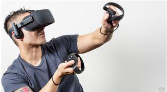
The final version of the Rift headset is, ultimately, a refined take on earlier prototypes, if one with improved ergonomics. It features two low-persistence AMOLED displays, an IR LED constellation system for 360-degree head tracking, built-in VR audio system and "high quality" internal microphone.
