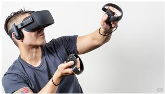
The final version of the Rift headset is, ultimately, a refined take on earlier prototypes, if one with improved ergonomics. It features two low-persistence AMOLED displays, an IR LED constellation system for 360-degree head tracking, built-in VR audio system and "high quality" internal microphone.
