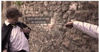
The concept behind the Maguss Wand is actually fairly simple. The wand carries motion sensors and an IR LED, while the badge holds an IR receiver. Users cast "spells" by waving the wand in various patterns picked up by the badge. In turn the badge communicates with the mobile app to keep track of duels and even provide sound effects.
