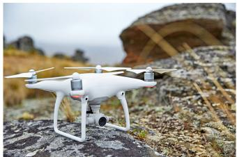
The obstacle sensing system involves a combination of two front-facing cameras and software allowing the drone to, well, spot and avoid objects. Thus the Phantom 4 can either automatically fly around obstacles or slow down to a hover if it cannot work out an alternative route.
