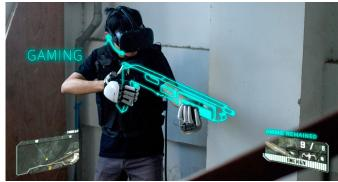
The Dexmo fits the hands like a glove, and tracks 11 degrees of freedom of motion. It applies force to the fingers when one is manipulating a virtual object, imitating the different levels of pushback provided by different objects in real life. As such, picking up a rubber duck in VR should feel different than, say, grabbing a brick.
