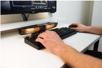
The Heatbuff uses infrared as a "no-burn technology" in order to keep fingers toasty, all while not melting keyboards or mice down. The actual device is around 38cm wide, and features twin heaters one can adjust and angle from the centre to customise the amount of heat provided.
