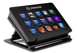
The Stream Deck connects to PCs via USB 2.0 and essentially is a miniature TV studio control board. Each of the 15 buttons has a tiny LCD display, allowing customisation with different icons for different functions. In total the Stream Deck handles up to 210 actions per configuration, since one can organise shortcuts into folders with the companion Stream Deck app.
