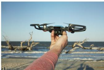
The miniature drone weighs 300g, and carries enough battery power to fly for 16 minutes. It can also shoot HD video and 12MP photos, has a 2-axis gimbal camera sabiliser, 3D sensing camera, GPS/Glonass and on-board software to mitigate shake and shutter roll. That said, what makes it really interesting is the aforementioned gesture control, allowing users to end the drone overhead and take a photo without need for a controller or app.
