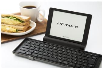
Essentially a miniature word processor, the Pomera on offer in our part of the world is just one of a line of such devices that has been available the land of the rising sun since 2008. It features a 6-inch elnk display hidden within a tri-fold keyboard complete with "generously sized" keys set in a Japanese layout.
