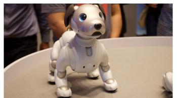
First seen back at CES 2018, the latest version of the Sony robot puppy promises to be far more advanced than the original 1999 Aibo. The head, chin and back carry touch sensors, allowing it "feel" pets, 22 actuators drive movement and the nose houses a camera allowing it to recognise family members. OLED panels allow for more expressive eyes, while a camera on the back allow it to navigate to its charging station, Roomba-style (with a single charge powering up to 2 hours of robot dog use).
