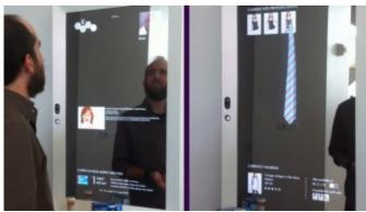
The New York Times R&D Lab combines a reflective LCD display, a Microsoft Kinect and the NYT.com APIs and creates a "Magic Mirror" ideal for bathrooms of the future.
